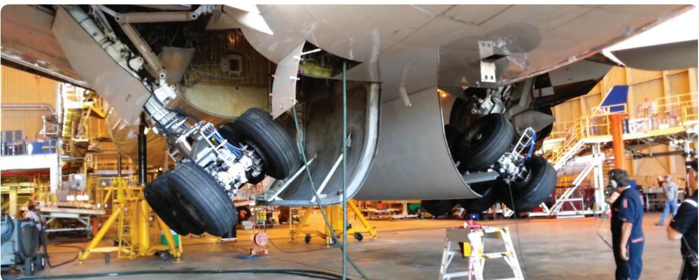
Figure 1.6 – A retraction test done after the plate was fitted as opposed to prior, would have prevented damage from this accident
