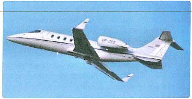
Figure 2-20. Winglets help reduce induced drag.
