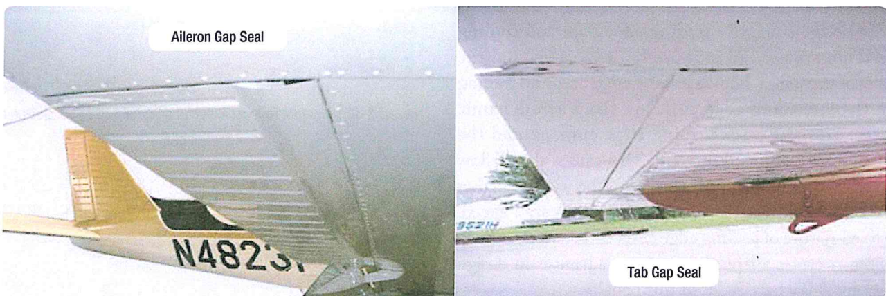
Figure 3-20. Gap seals promote the smooth flow of air over gaps between fixed and movable surfaces.
