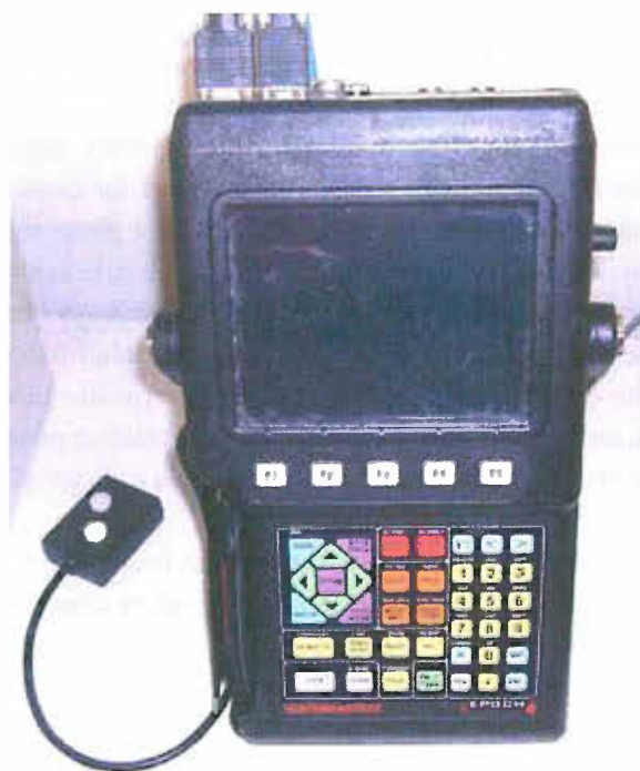
Figure 3-28. Pulse echo test equipment.
