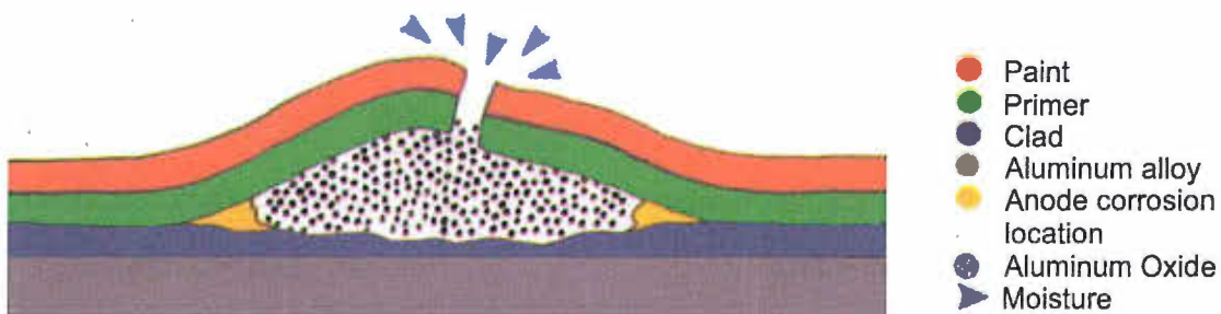
Figure 4-8. Filiform corrosion.
