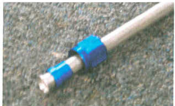
Flared tube assembled with sleeve and nut.
