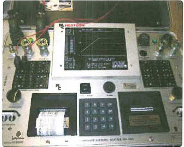
Figure 3-42. Heat bonder equipment.
