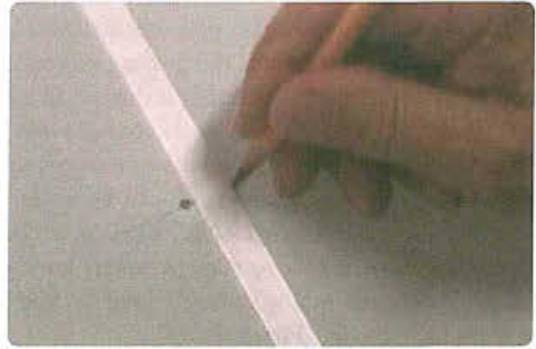
Figure 3-153. A premarked location for a lacing hole, which is punched through the fabric with a pencil.
