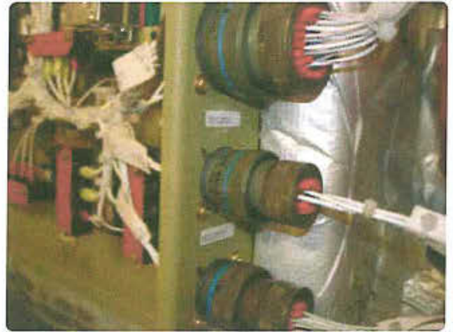
Figure 11-52. Connector arrangement to avoid wrong connection.
