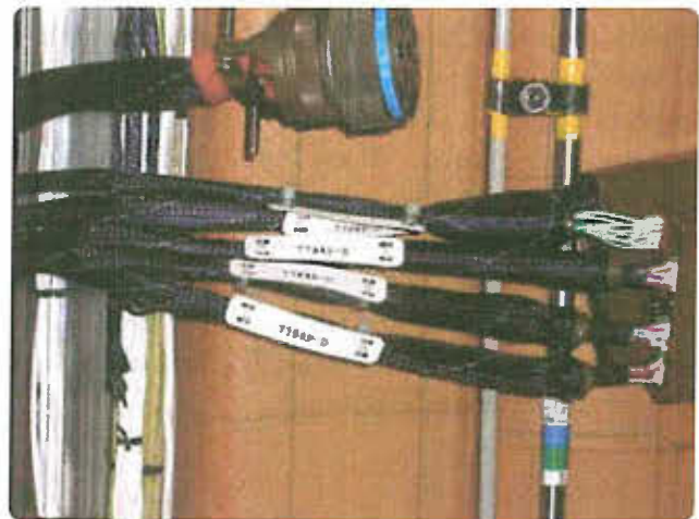
Figure 11-18. Alternate method of identifying wire bundles.
