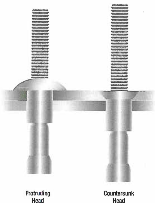
Figure 5-42. Self-plugging (friction lock) rivets.
