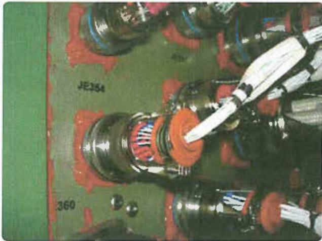
Figure 11-53. Backshells with strain relief.
