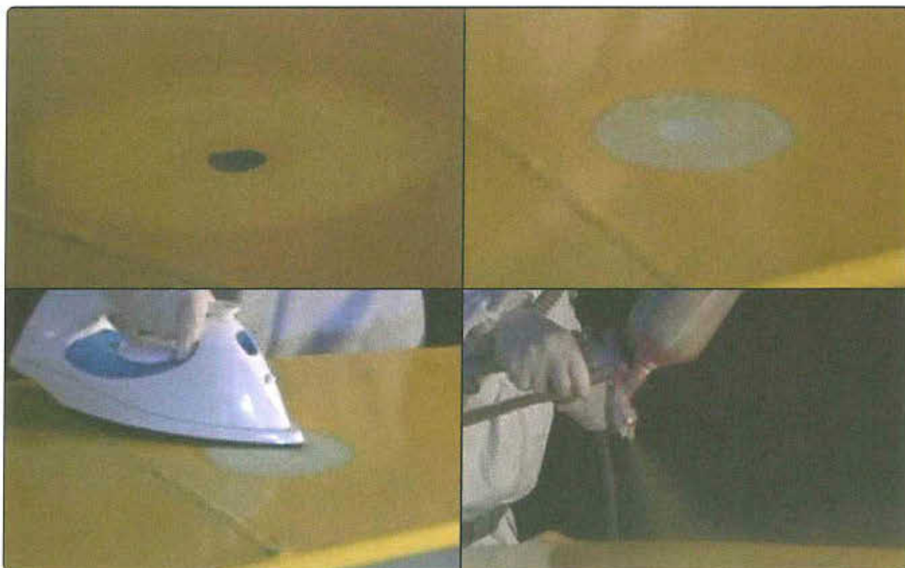
Figure 3-164. A patch over this small hole on a polyurethane top coat is repaired in accordance with the repair instructions in the STC under which the aircraft was re-covered. It requires only a two-inch fabric overlap and scuffing into the top coat before cementing and refinishing. Other STC repair instructions may not allow this repair.
