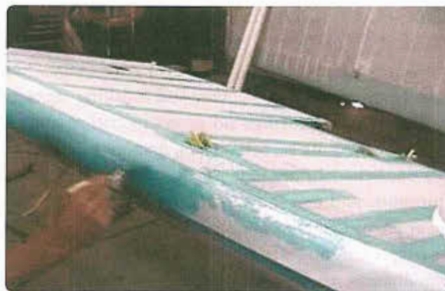
Figure 3-162. Cement is brushed through a four-inch tape during installation over the fabric seam on a wing leading edge. Two-inch tapes cover the wing rib and rib lacing.
