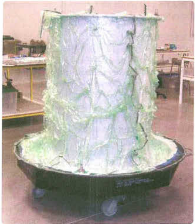
Figure 3-38. Bagging of complex part.
