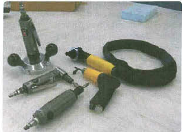
Figure 3-34. Air tools used for composite repair.
