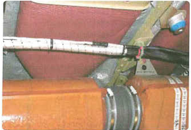
Figure 11-4. Shielded wire harness for flight control.
