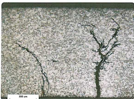
Figure 4-12. Stress corrosion cracking.
