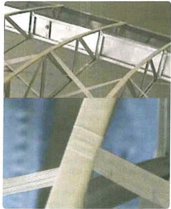
Figure 3-148. Anti-chafe tape is applied to all features that might cut or wear through the fabric.
