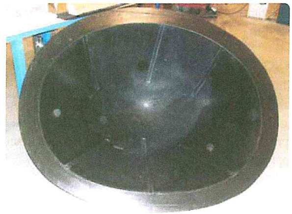
Figure 3-70. Radome repair tool.
