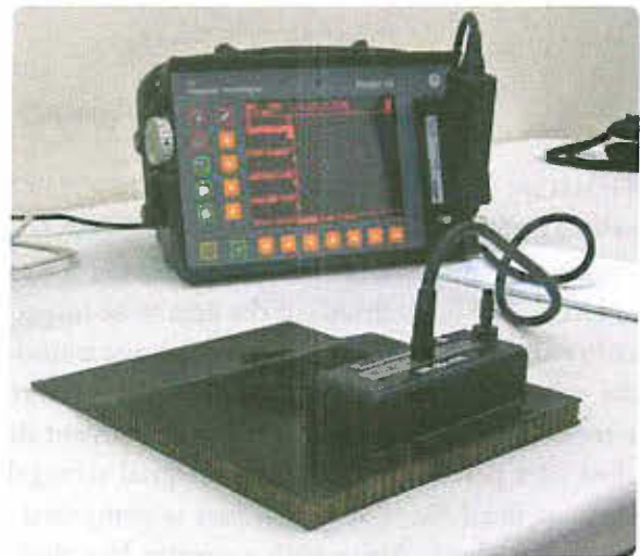
Figure 3-30. Phased array testing equipment.
