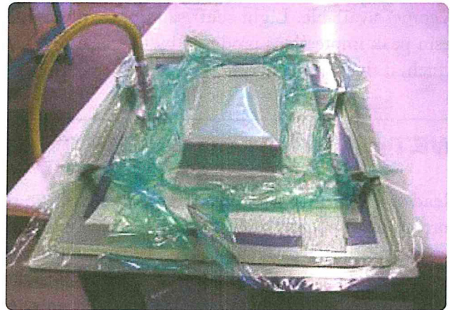
Figure 3-50. Vacuum bagging of contoured part.
