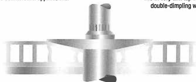
156° Countersunk NAS 1097 A large diameter, shallow countersunk head providing wide area for honeycomb applications.
