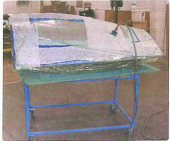
Figure 3-54. Envelope bagging of repair.
