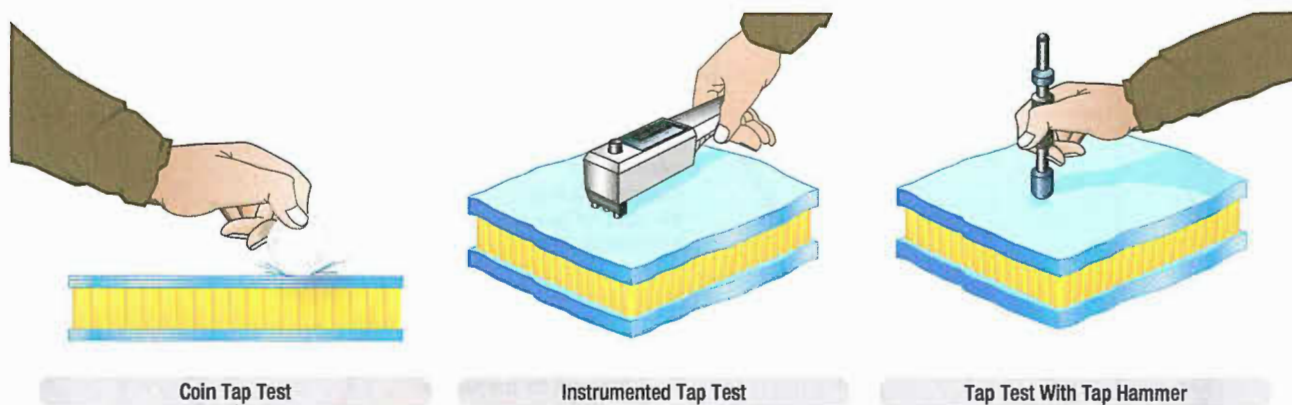
Figure 3-57. Tap testing techniques.
