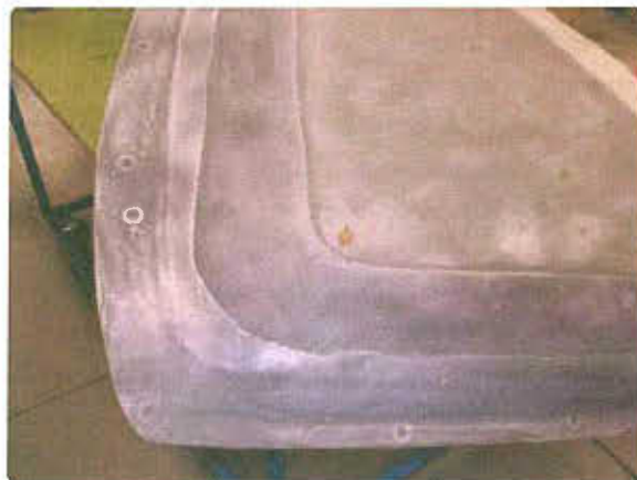
Figure 3-11. Aluminum mesh lightning protection material.
