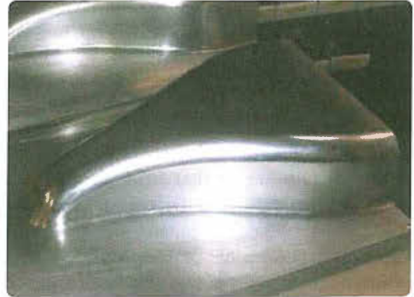
Figure 3-36. A mold of an inlet duct.
