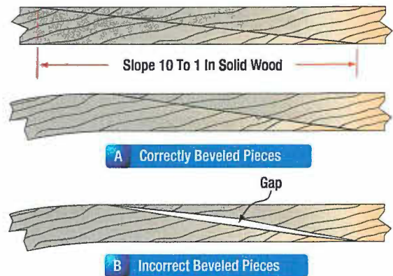
Figure 3-119. Beveled scarf joint.
