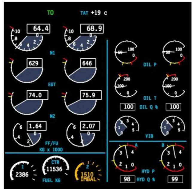
Figure 1-9. EICAS engine display format.
