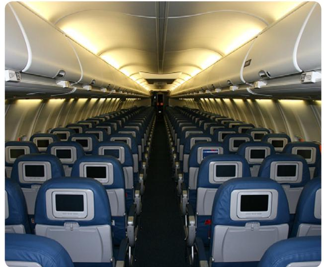
Figure 10-9. Panasonic IFE system installed on a Boeing 737-800.
