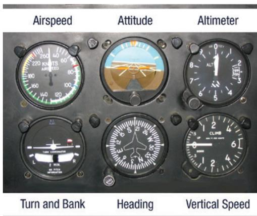
Figure 1-1. Basic Analog Cockpit Flight Instruments.
