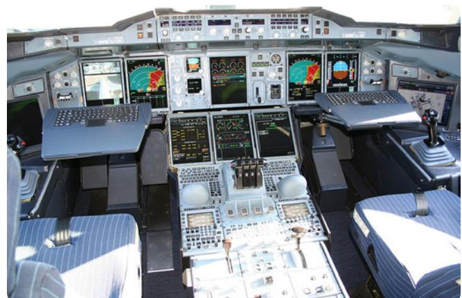
Figure 1-2. Airbus A380 EIS with 8 Large LCD Displays.
