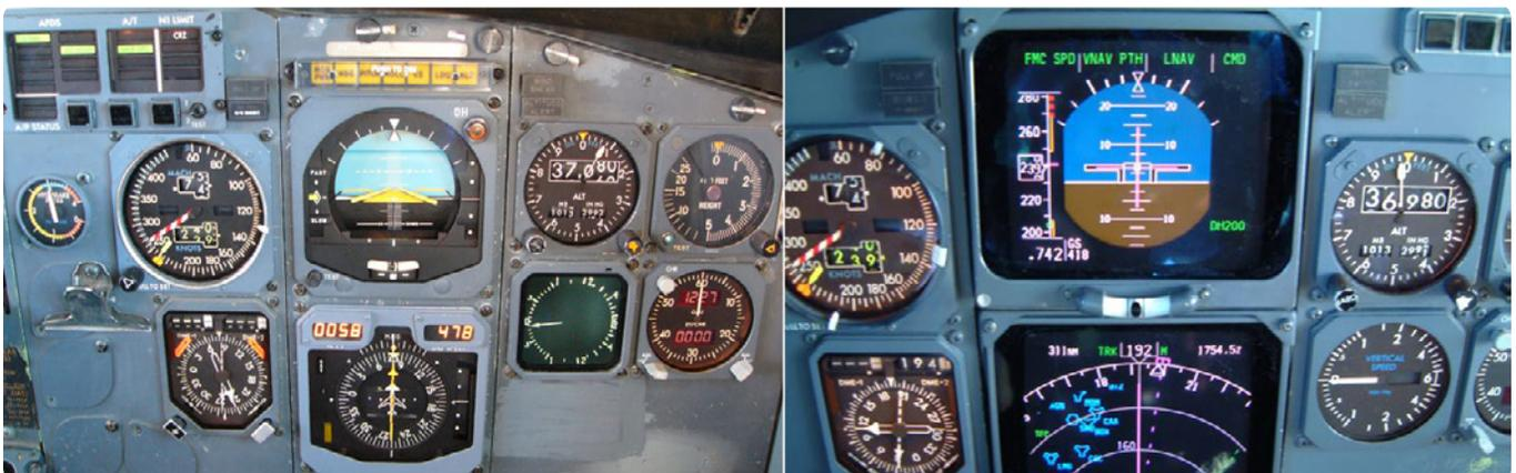
Figure 1-3. Equivalent Electromechanical Flight and Navigation Instruments on the left.
