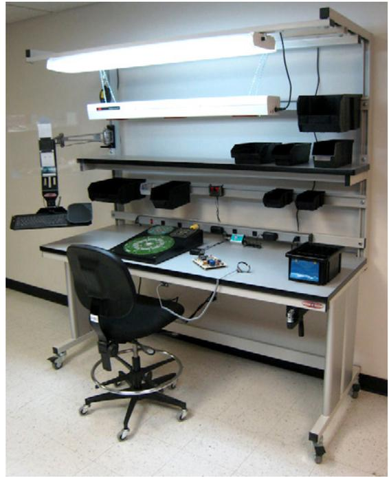
Figure 12-4. Static-safe workstation.
