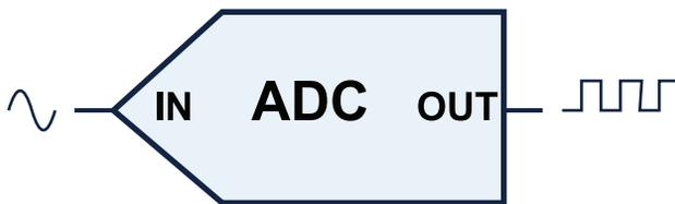
Figure 3-3. Symbol for an analog to digital converter.
