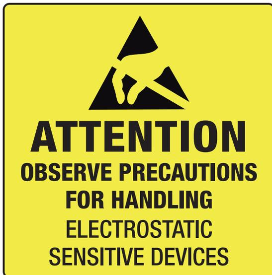
Figure 12-3. Warning sign for an ESD controlled area.
