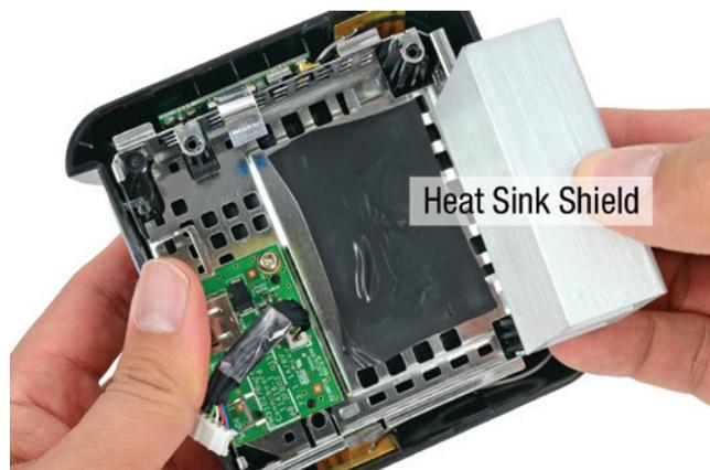
Figure 14-5. Heat-sink shield acts as a faraday cage to block electromagnetic emissions.
