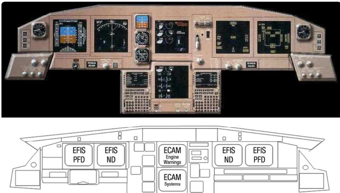
Figure 1-6. Boeing 777 Electronic Instrument System has 6 LCD Displays.
