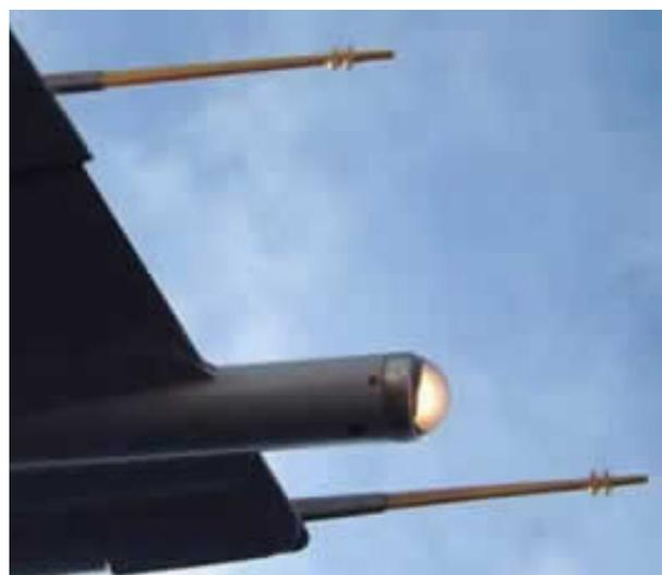
Figure 14-4. Static wicks on Boeing 737 wing.
