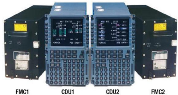
Figure 15-10. FMS Block Diagram (left) and FMS LRUs (right).
