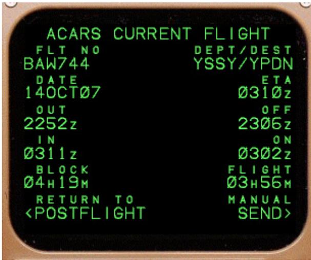
Figure 15-6. Typical ACARS display format.
